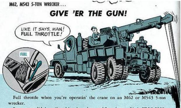
Some guys didn't realize this when they read Step 4, page 51, in TM 9-2320-211-10. So the hydraulic pump didn't run fast enough to open the vanes all the way. The vanes got to chattering, and pretty soon the pump went bust.
